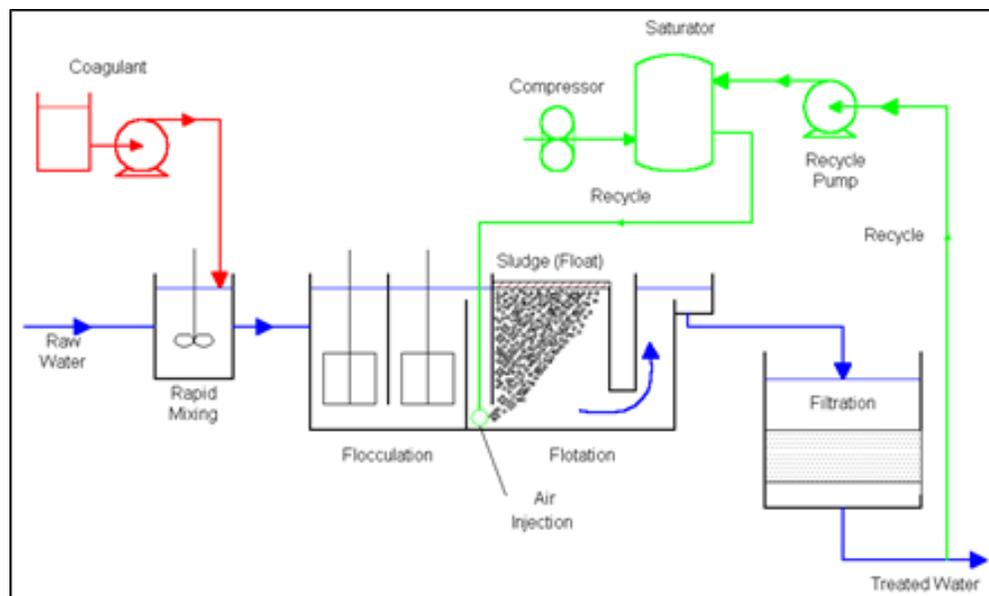
Figure 4.2: Schematic Diagram of DAF Process
