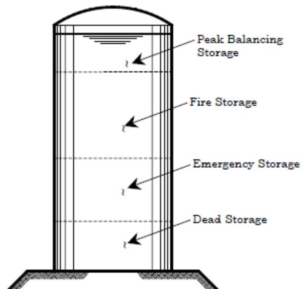
**Emergency storage** is the volume of water in reserve to cover maintenance shut-down or emergency situations such as source of supply failure or other major incidents. A standard method of calculating this volume is 25% of the sum of the peak balancing volume and fire storage.
