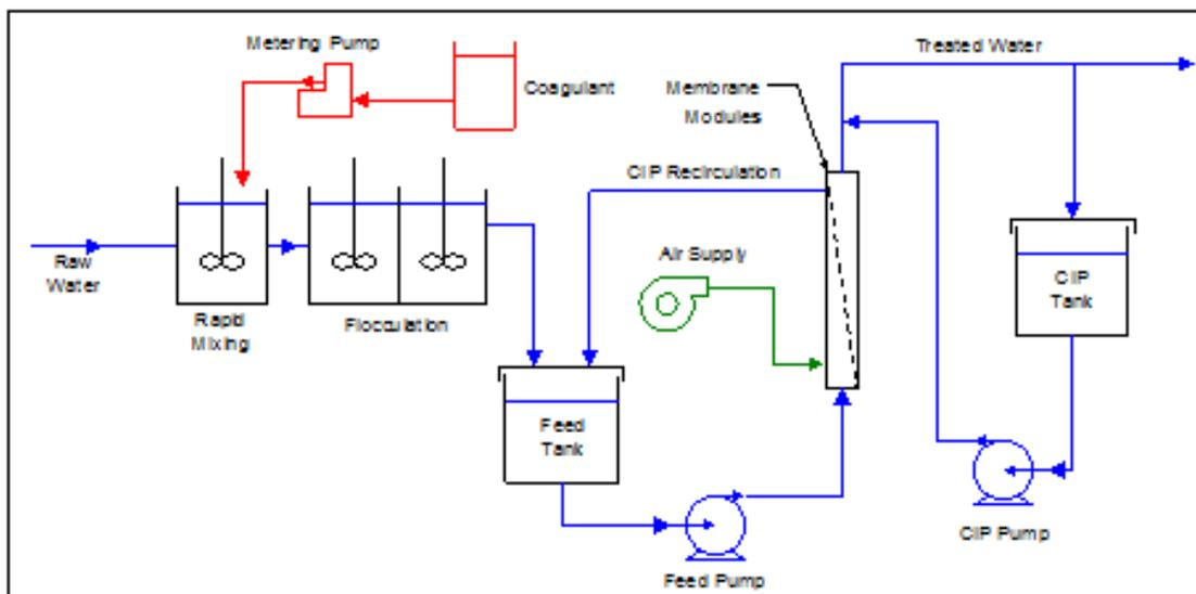
**Figure 4.3: Schematic Diagram of Ultrafiltration Process**
